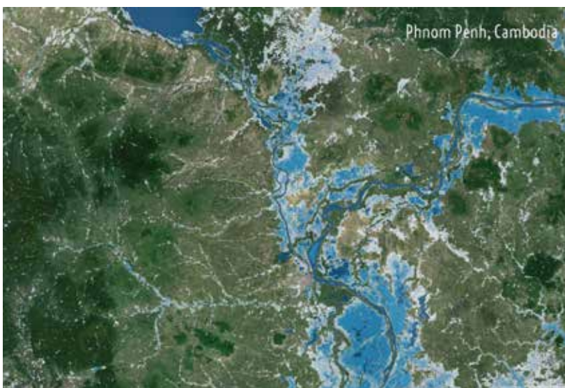
Figure 2. Part of a 90m resolution flood hazard map produced by the University of Bristol, UK, and SSBN Ltd. by downscaling from a 1km resolution global hydrodynamic model. The map shows the area at risk from fluvial and pluvial flooding with an annual probability of 0.01 (1-in-100-year return period) for Phnom Penh, Cambodia.
