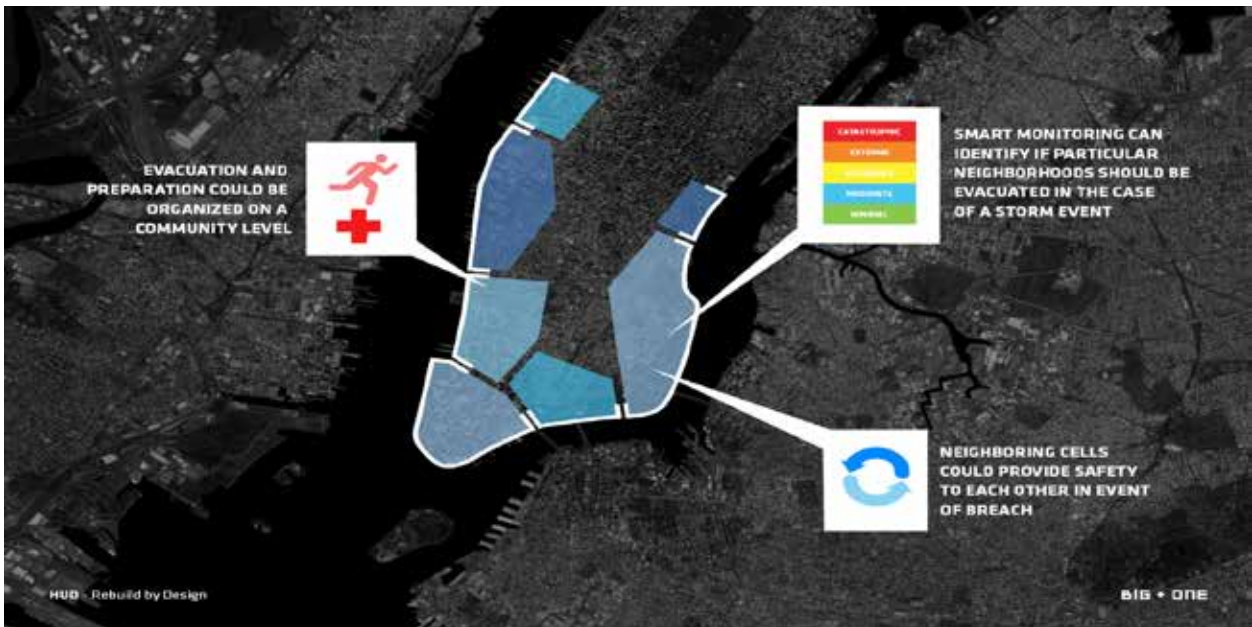
Figure 4. Compartmentalized flood defense design for Manhattan, New York City. Each compartment enables flexibility because it encourages a design and risk mitigation plan relevant to that community.
