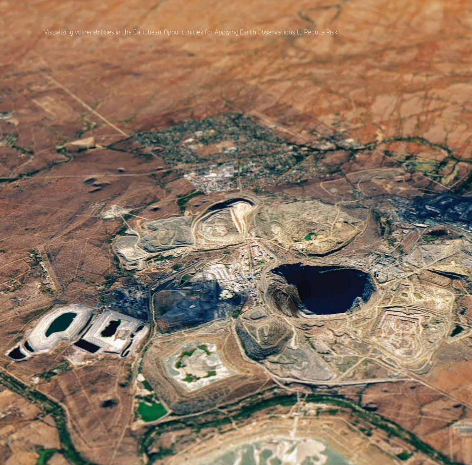
▲ Figure 1. The Palabora mining pit has been growing steadily in size since 1965, and is the largest open mine in South Africa. Operations have moved underground leading to structural collapses and damage to nearby roads, power and water lines, and other infrastructure. Using LandSat and SRTM data, NASA researchers are using data to improve the understanding of how continued underground mining will deform the land surface and lead to further collapse and impact to surrounding communities like Phalaborwa, in the future.
