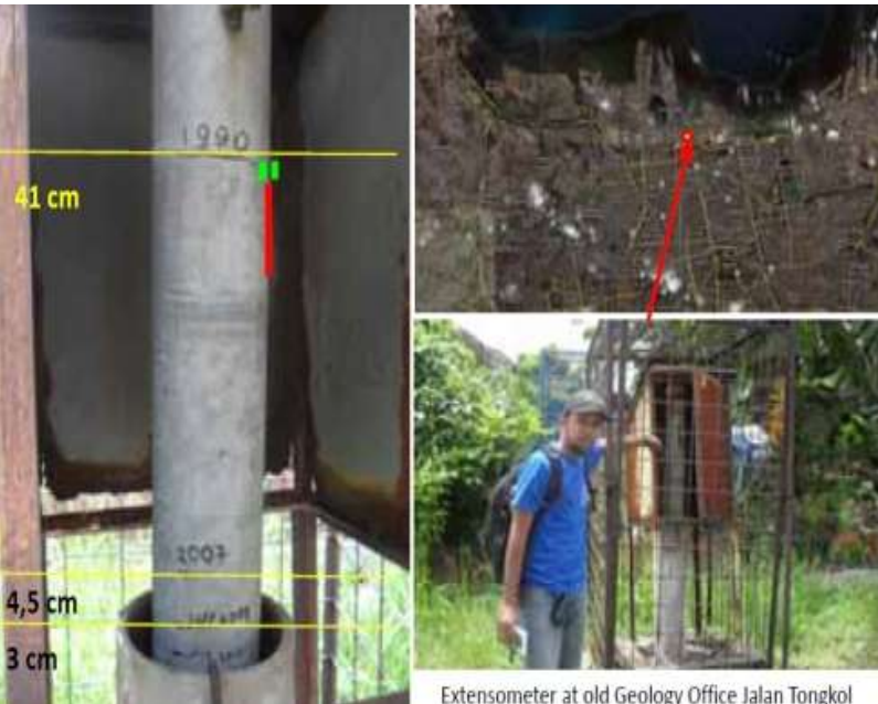
Extensometer at old Geology Office Jalan Tongkol
